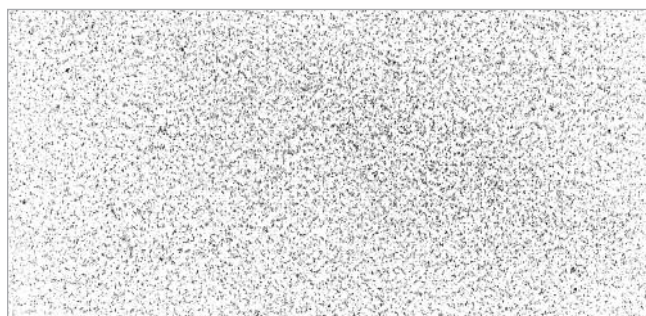
Wire side: Finer, regular pattern of the wire mesh
