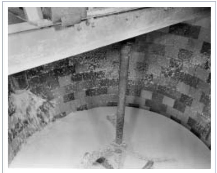
*Pulp is fed into a holding tank where it will get mixed with more water and sent to the paper machine.*
